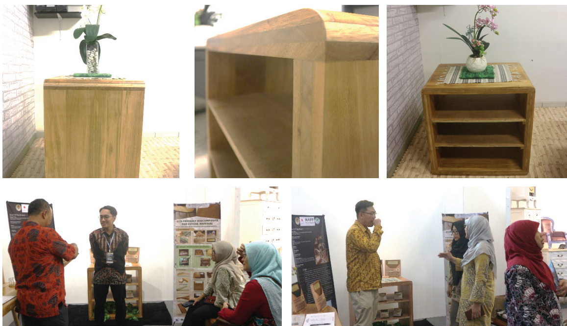
Figure 68 Shelf made from mahogany-sengon-mahogany CLT
