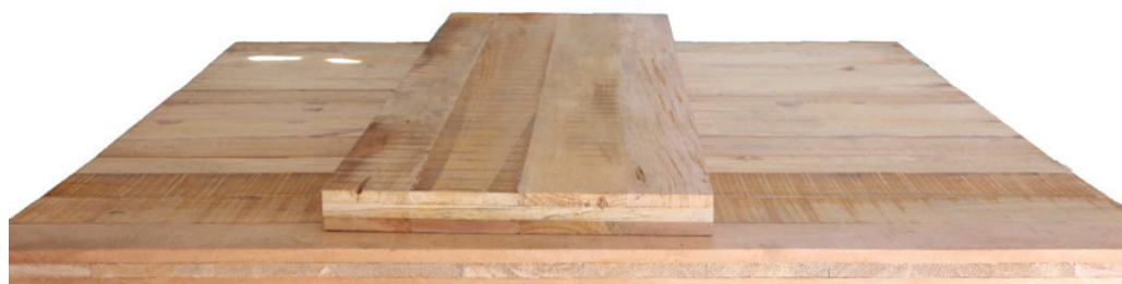
Figure 66 Cross-laminated timber (CLT) mahogany-sengon-mahogany
